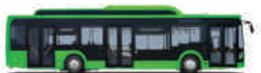
AVENUE LOW-FLOOR CNG L: 11.995 m, H: 3.540 m (with tanks)
