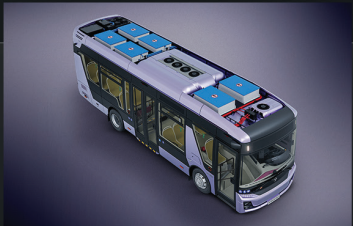
8x48 kWh TemsaTech Batteries 600km Range
